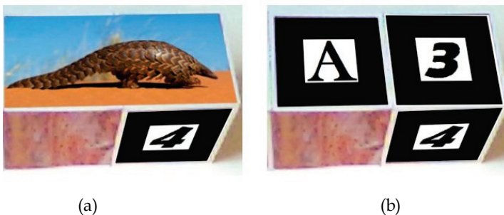
Fig. 4. a) AR game. A scaly anteater appears on the cubes as an augmented image. b) The same cube as in Figure 4.a., but without an image
